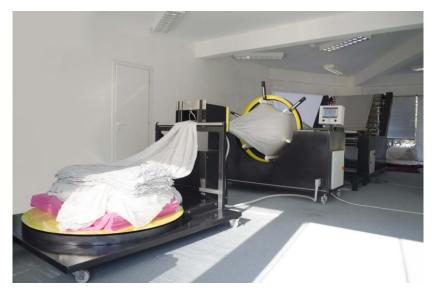
The only needed data for input are the percentage of the spirality (determined by tumbler test), the width of the fabric and the direction of rotation.
